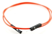
Figure 3. A male-to-male jumper wire. It can be easily connected to the breadboard and the Arduino pins (image courtesy of Sparkfun).
